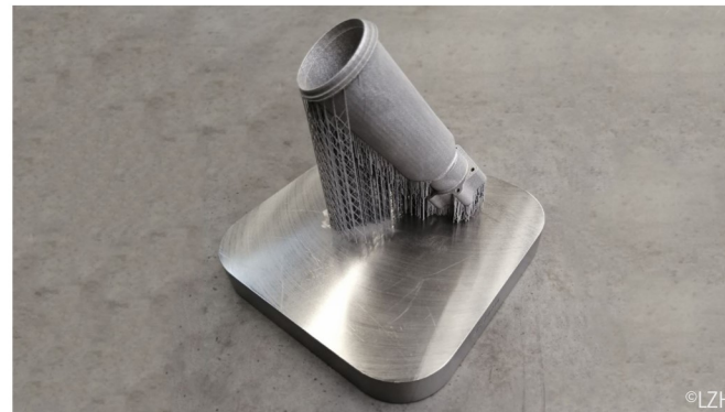
Simplifying structures: One part instead of three
