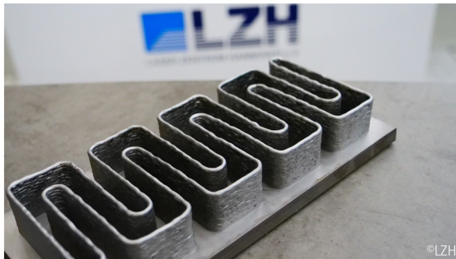
Manufacturing using coaxial laser-wire deposition welding
